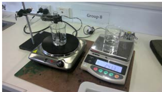
Comparison of the specific heat capacities of iron and its alloys - alloys have more specific heat capacity.
